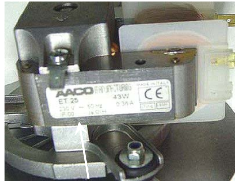
fig.2 — Replacement AACO Venter Motor
