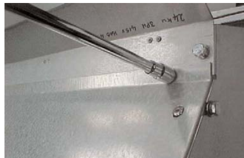
fig.4 – Access plate securing bolts
