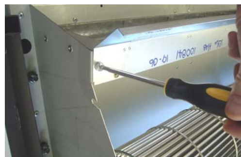
fig.5 – Element assembly securing bolts.
