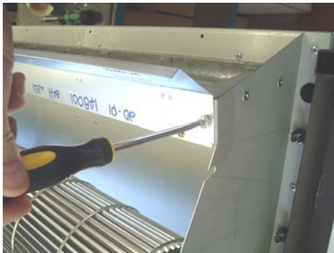
fig.7 – Element assembly securing bolts.
