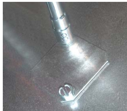
fig.20 - fixing blanking plate over LC3 capillary hole
