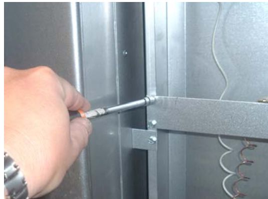
fig.21 - position new limit stat bracket
