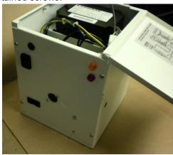
8) Finally, replace the wiring diagram on the door with the one supplied 900224-WD.
