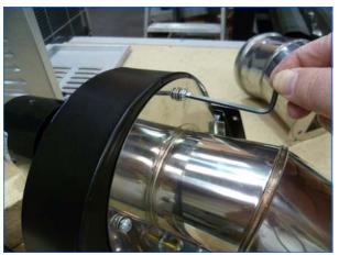
Fit the fan outlet to the fan using four set pins/ washers as shown.
