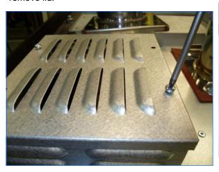
Remove the three air inlet box retaining screws, (retain for future use) then remove box taking care not to damage the foam gasket. (See next photo).
