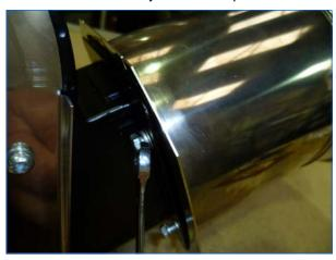
Fit the new fan assembly and red gasket to the air curtain using the four existing screws. Refit the vacuum tube, then connect the 3 pin plug for the power supply.
