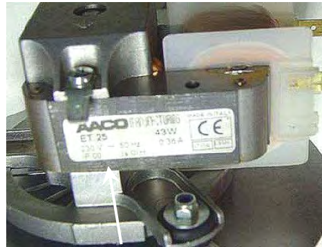
fig.2 - Replacement AACO Venter Motor
