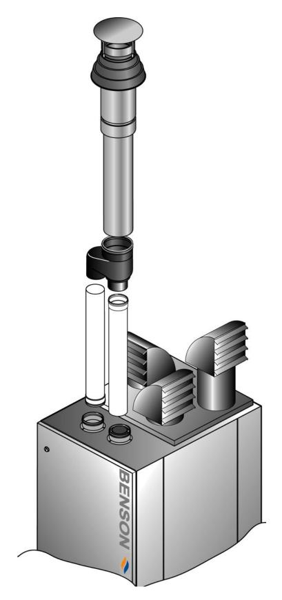
$B_{22}$  Single flue Option In this configuration the heater is connected to a single flue pipe to discharge the products of combustion outside the building either through the roof or through a wall. The air for combustion is taken from inside the building.
