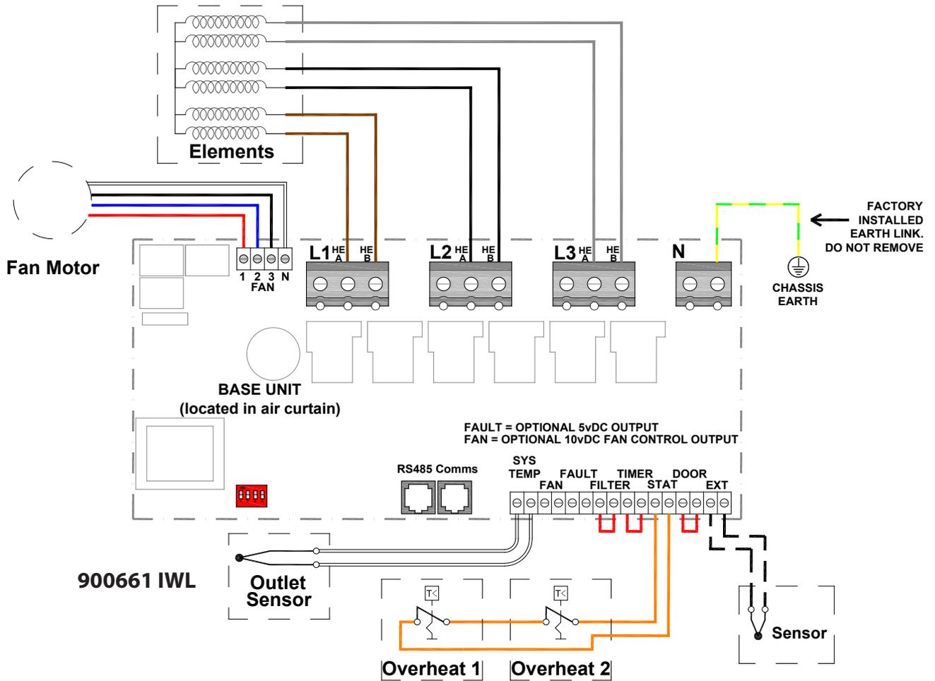
The element output is connected to the right and left side of each terminal block marked "HE A" & "HE B"
