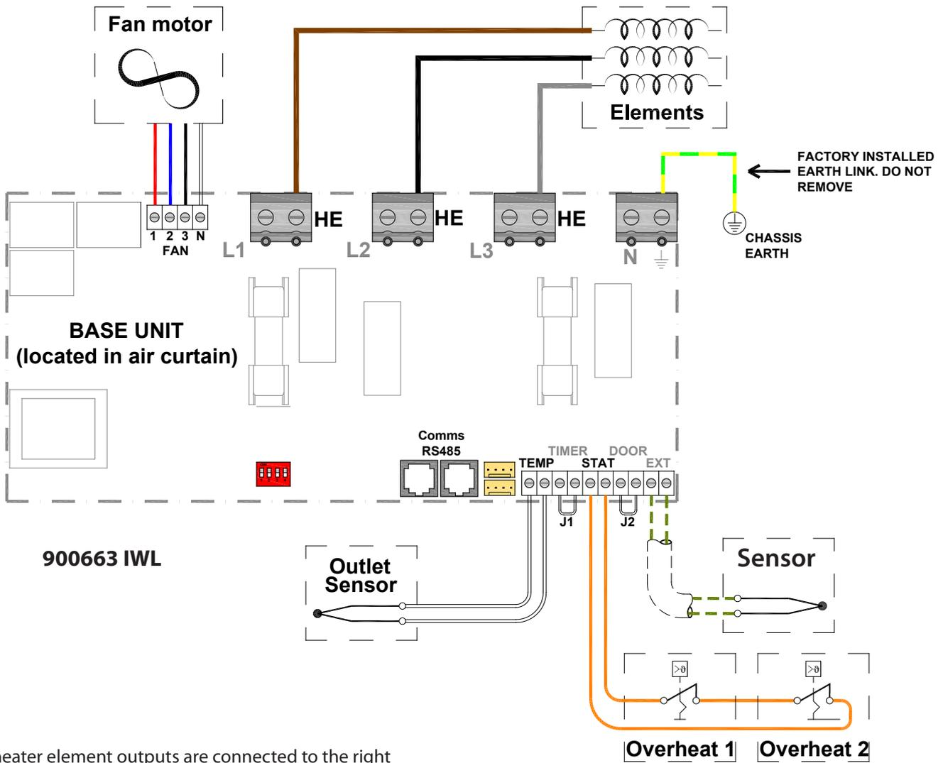
The heater element outputs are connected to the right hand side of three terminal blocks and are marked 'HE'. (See below).
