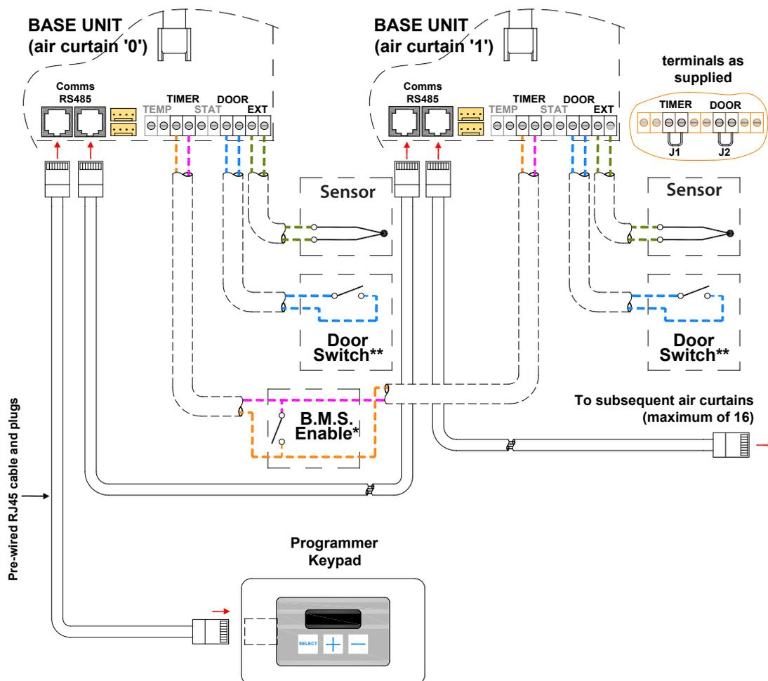
This diagram refers only to the wiring of 2 or more networked air curtains. (maximum 16 air curtains per control panel). For mains wiring refer to section 4 of this manual 'installer wiring details'.
