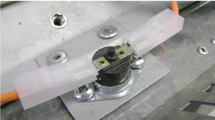
Fig. 13. Thermal Cut-out
