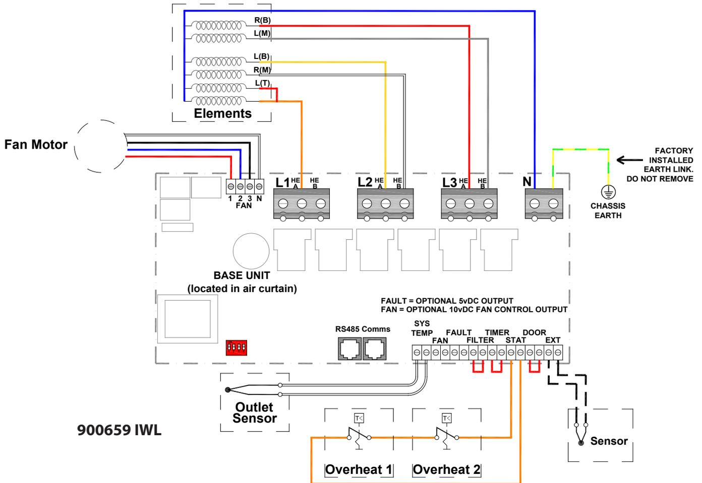
The element output is connected to the terminal blocks marked "L1 A", "L2 A&B", L3 A&B"
