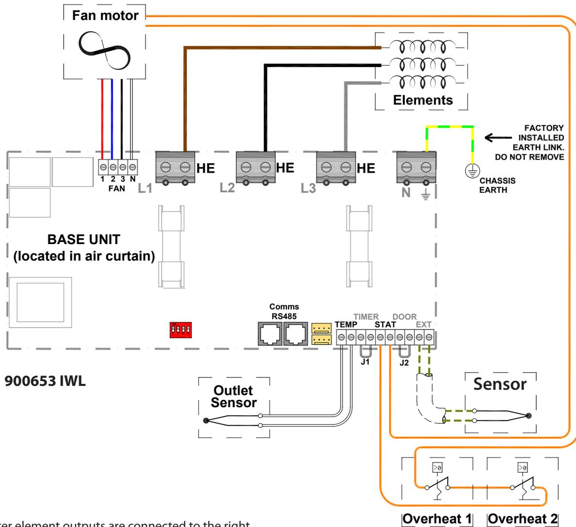
The heater element outputs are connected to the right hand side of three terminal blocks and are marked 'HE'. (See below).
