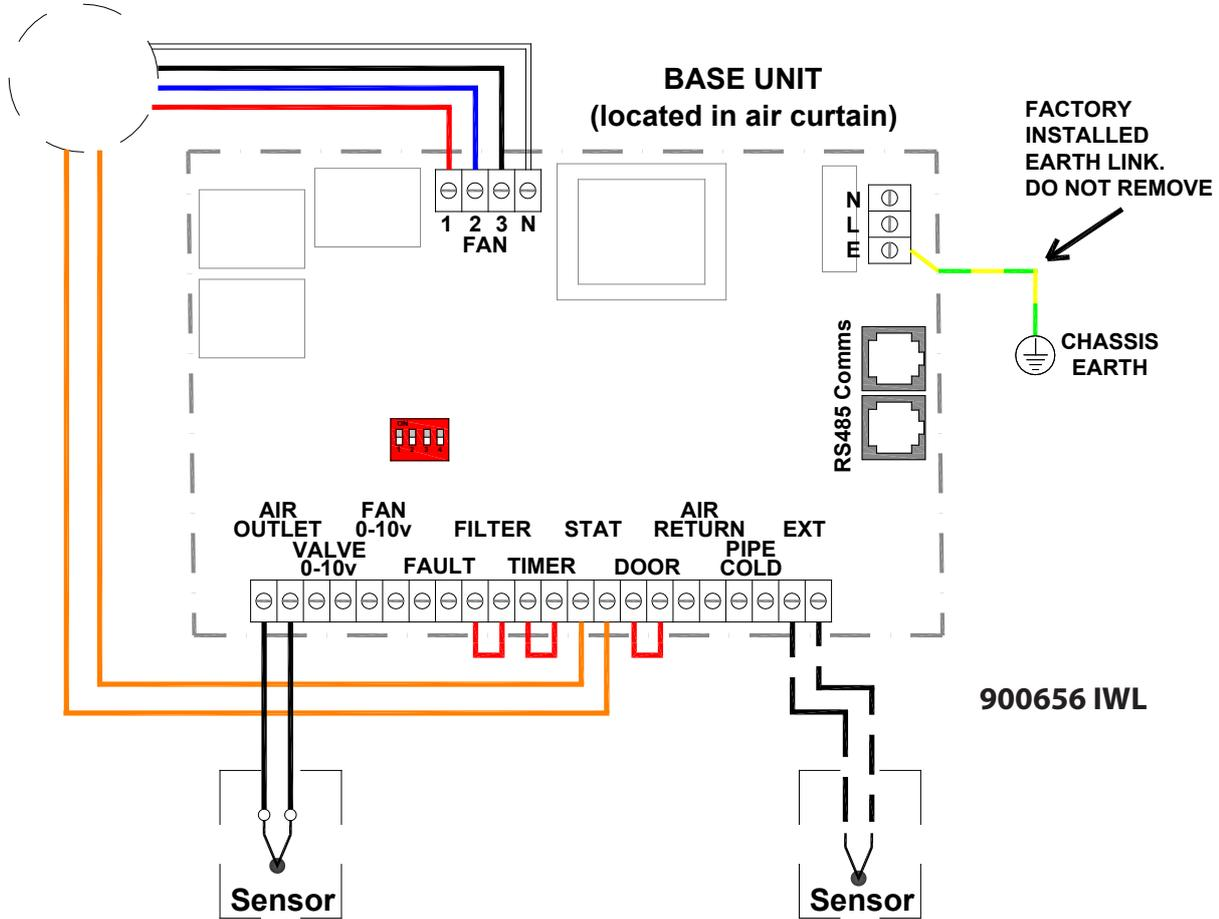
The fan output is connected to a 4 way connector marked "Fan 1,2,3 & N"
