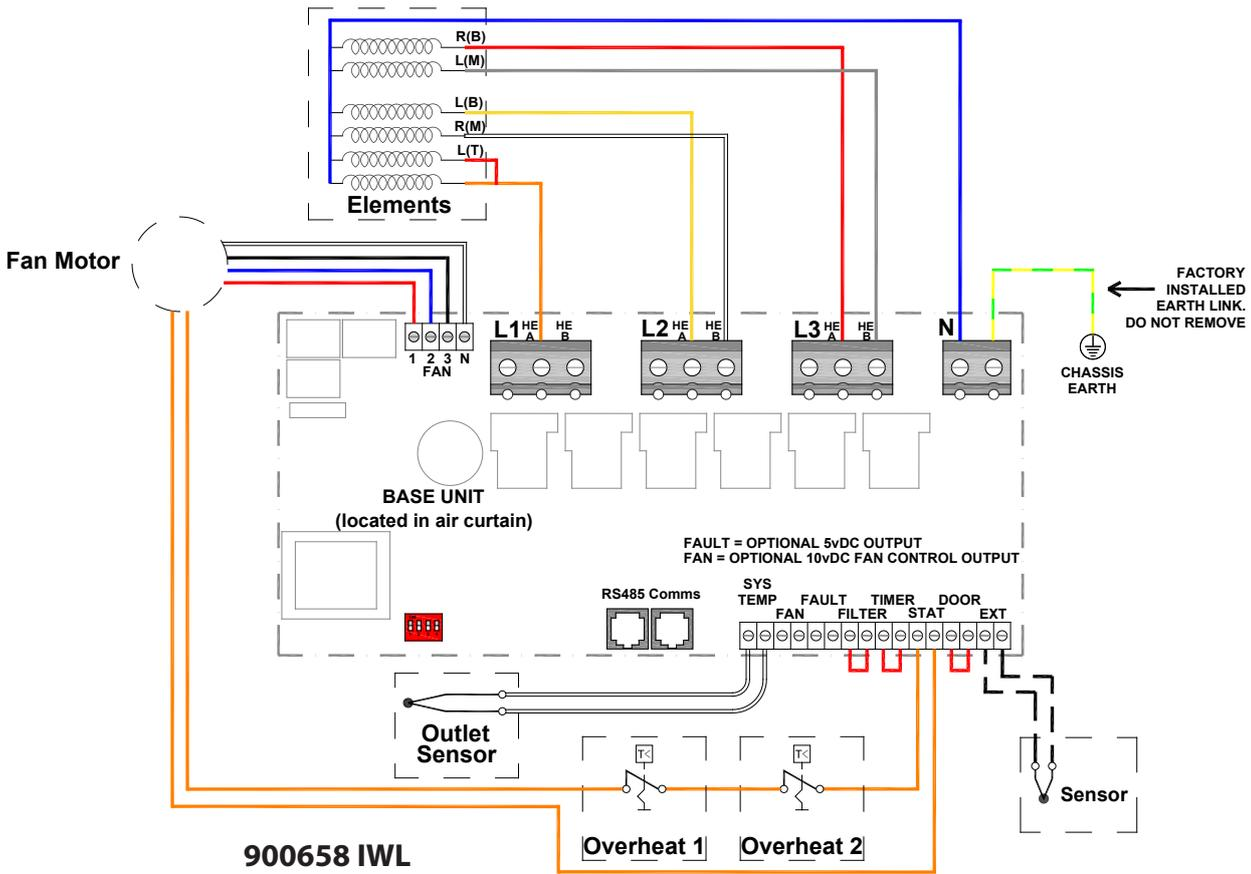
The element output is connected to the terminal blocks marked "L1 A", "L2 A&B", "L3 A&B" "N"
