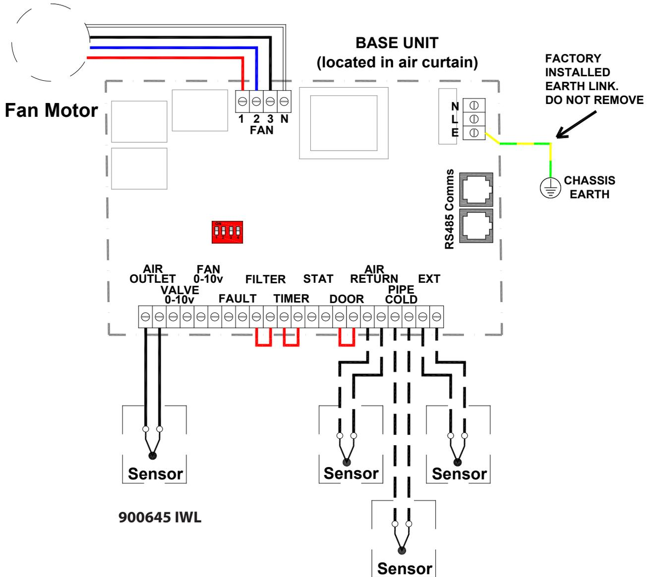
The fan output is connected to a 4 way connector marked "Fan 1,2,3 & N"
