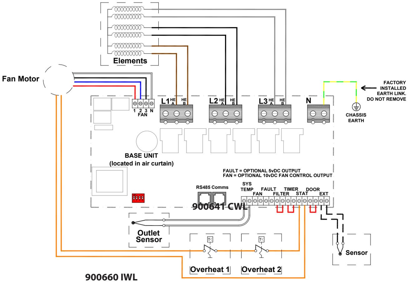
The element output is connected to the right and left side of each terminal block marked "HE A" & "HE B"
