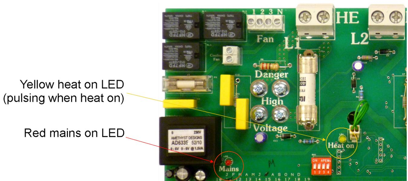
Note: Standard controller LEDs have the same function and are in similar positions on the PCB.
