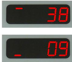
These show the permissible upper and lower limits for setting the external temperature sensor set point. This is useful for allowing the end user limited control over this setting. The maximum (default 35°C) may be set anywhere between the current minimum and 50°C, and the minimum (default 16°C) may be set anywhere between 3°C and the current maximum.
