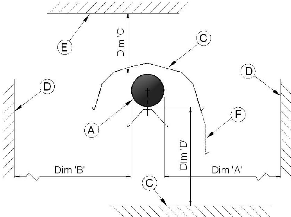
Distance from combustibles (distance from heat source that will produce a 50°C rise in temperature above ambient of a black surface) **A** Radiant tube; **B** Standard reflector; **C** Combustible material underneath; **D** Combustible material on side; **E** Combustible material above; **F** Perimeter reflector;
