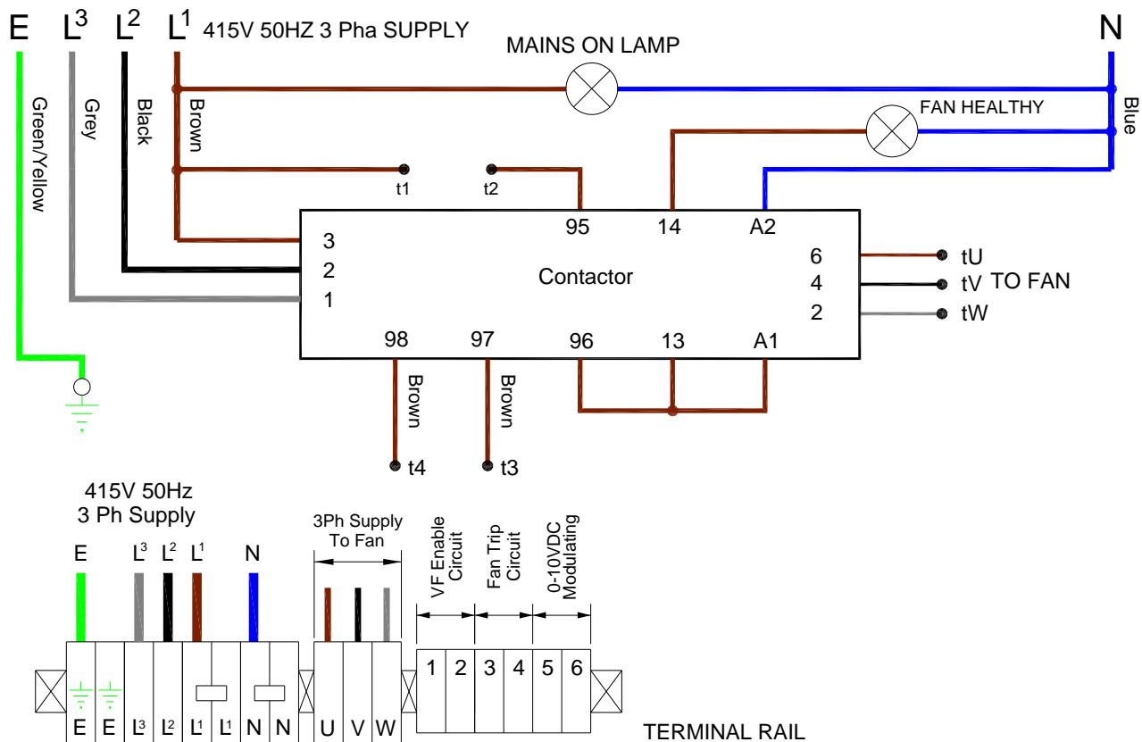
**Figure 4.I. NRV Schematic interconnecting wiring. B80, B160 and B300 three phase fans controlled by SmartCom3 via single phase Inverter panel. (single zone shown)**
