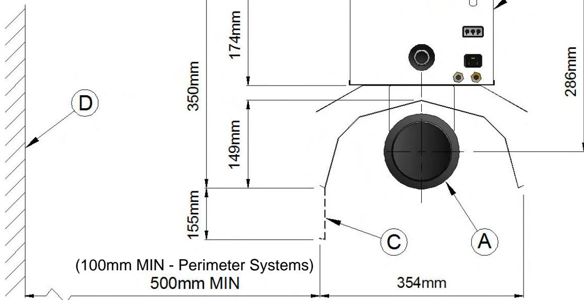
**Figure 1.b Clearance for servicing - distances to walls and obstacles above.**
