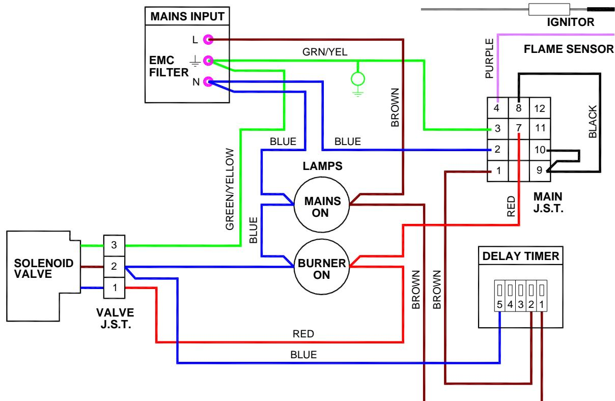
Figure 4.e. LR internal wiring diagram - End Vent Burner c/w N/O or N/C volt free Lockout contacts
