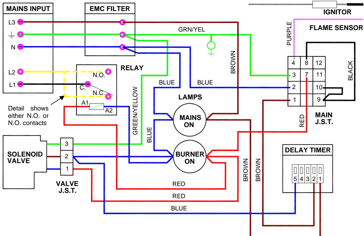
Figure 4.g. LR internal wiring diagram - End Vent Burner c/w 3 way solenoid valve
