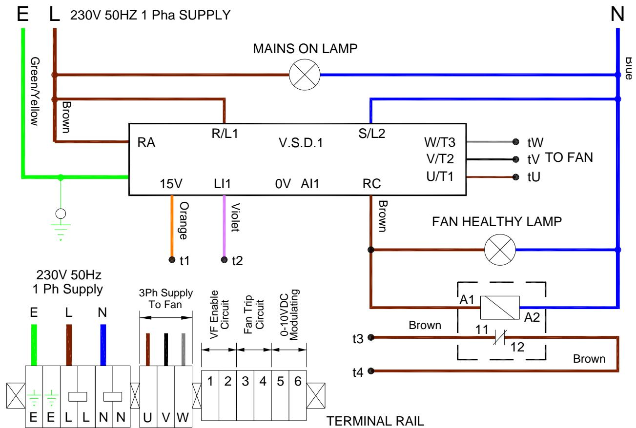
**Figure 4.k. NRV Local Relay Unit Internal Wiring Diagram for BH300 three phase fans**
