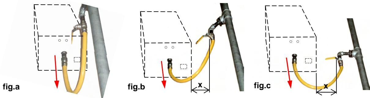
Depending on the specific installation, the flexible gas hose may be routed to the gas cock at any of the following angles in relation to the burner:
