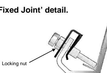
**⚠** Fully tighten these screws for **fixed joints**. Then secure with the locking nut.
