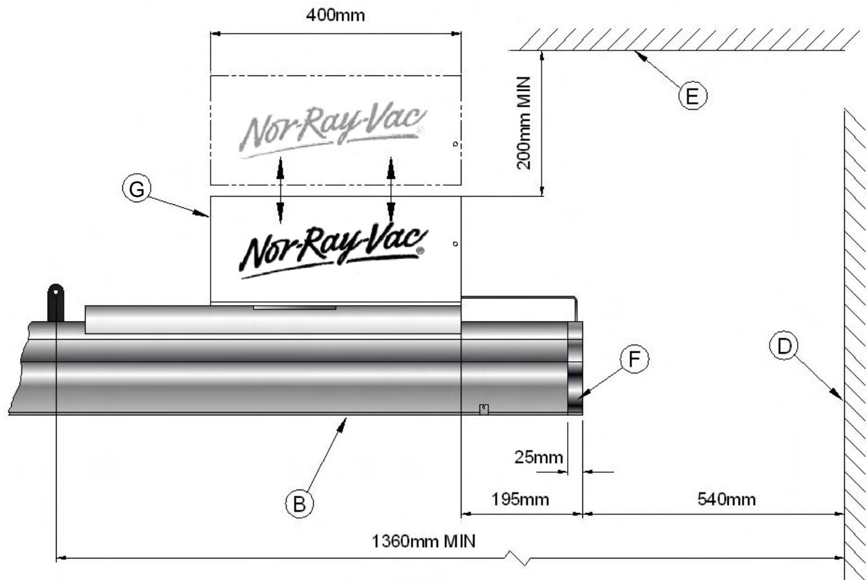
**Figure 1.c Clearance for servicing - distances to obstacles above.**
