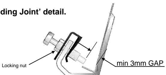
**⚠** Leave a minimum 3mm gap clearance between reflector and screws for a **sliding joint**. Then secure with the locking nut. The reflector overlap after each burner must be a 'sliding joint', to allow for thermal expansion.
