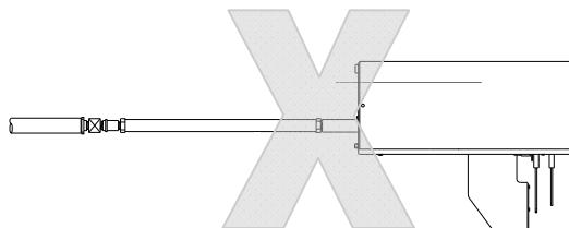
The methods shown in fig.f and fig.g are unacceptable, due to undue stress on the hose & fittings.
