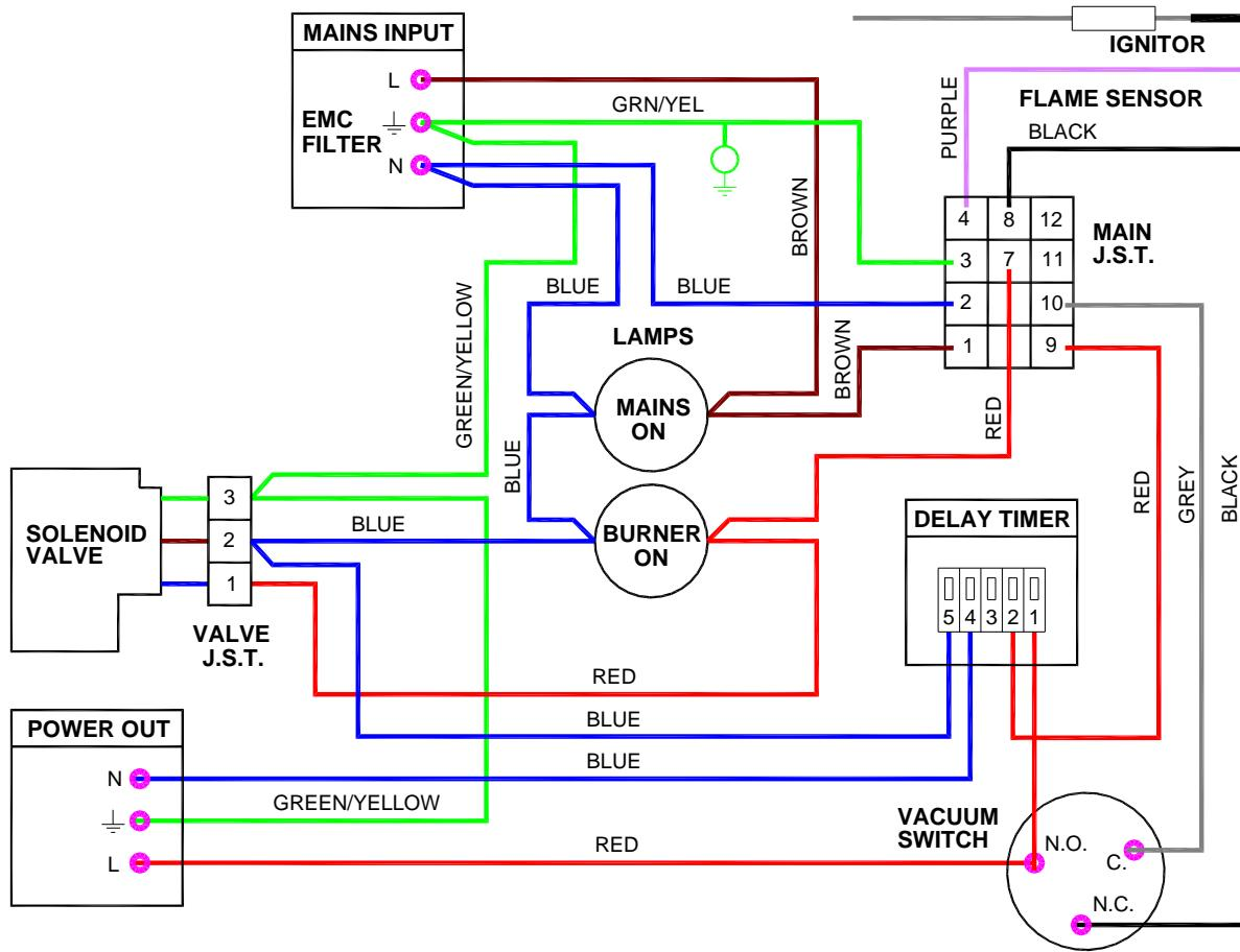
Figure 4.d. LR internal wiring diagram - In-line Burner (IL)
