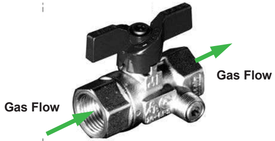
Figure 2. Correct orientation of Ball Valve
