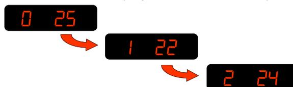
Any air curtain in the network can be accessed by pressing the
