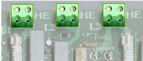
The heater element outputs are connected to the right hand side of three terminal blocks and are marked 'HE'. (See below).
