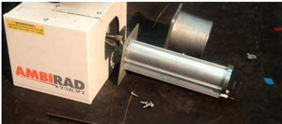
**Step 5:** The burner head can now be detached by disconnecting the impulse tube and the burner head wiring.
