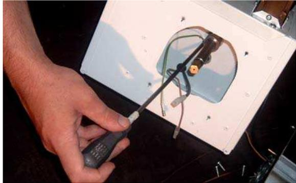
**Step 7:** Remove the four screws (arrowed) holding the rear burner plate in position.
