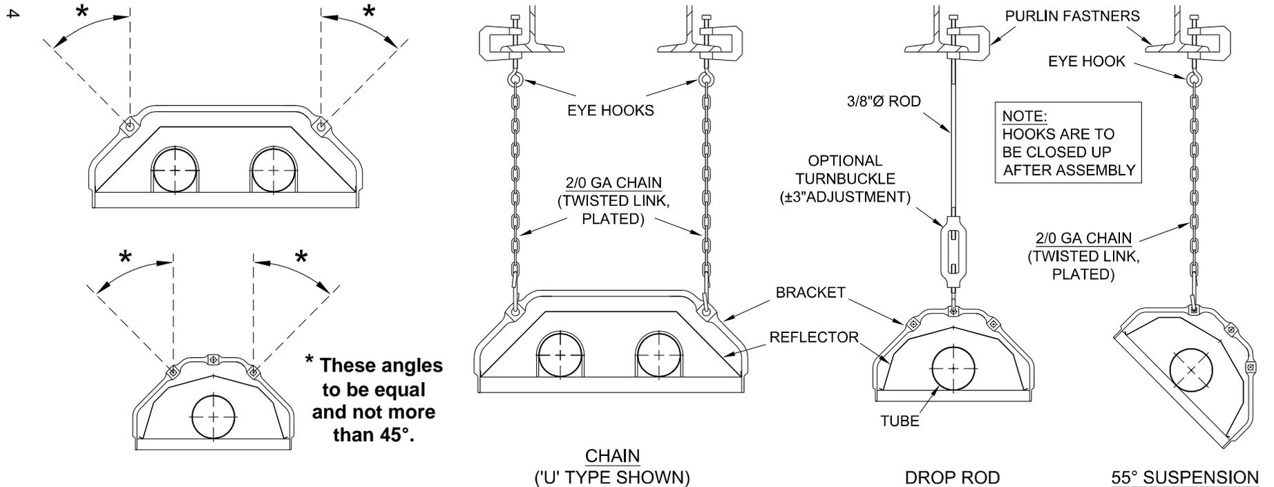
Figure 1. Recommended Methods of Heater Suspension.
