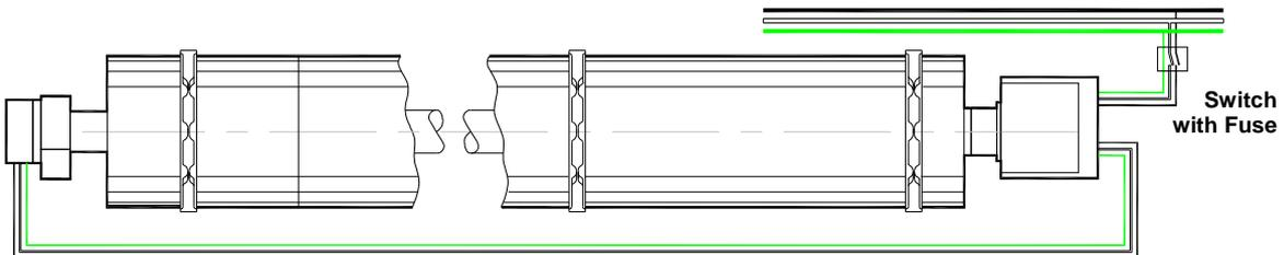
**Figure 5c. Single and Multiple Heater Installations 120V Control**
