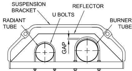
FIRST POINT SUSPENSION BRACKET TYPE B
