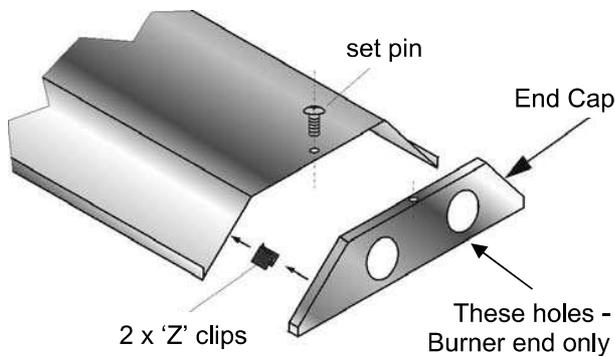
**On linear models only**, position ONE end cap beneath the reflector profile at the fan end with the end cap flanges facing inwards.
