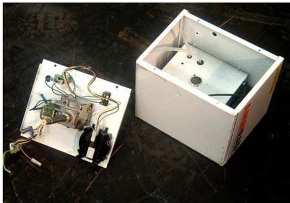
**Step 9:** The two screws retaining the gas valve can now be removed.
