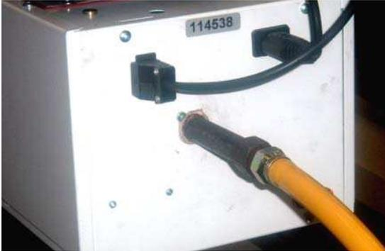
**Step 3:** Detach the gas supply as shown below, taking care to support the burner connection.
