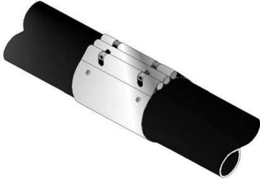
Slide the coupler over the tube ensuring that the rivet stop has butted up to the tube ends. Using an Allen wrench, tighten the pins.
