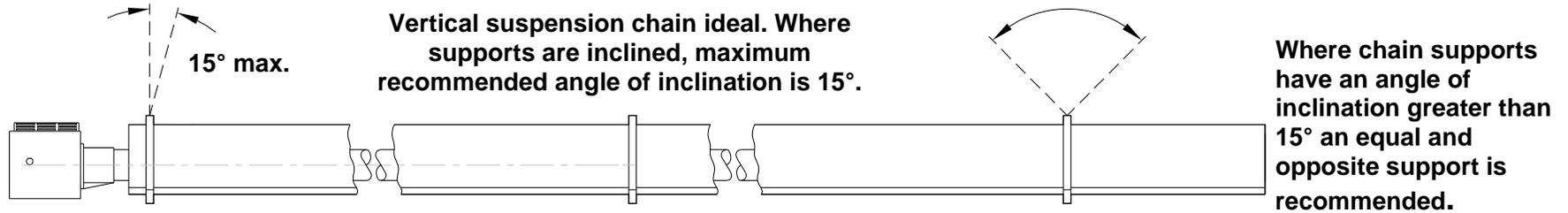
**ON U TUBE VARIANTS THE HEATER SHOULD SLOPE DOWNWARDS TOWARDS THE RETURN BEND AND ON LINEAR VARIANTS SHOULD SLOPE DOWNWARDS TOWARDS BURNER BY APPROX. 1/2" FOR BOTH HORIZONTAL AND WALL MOUNTED INSTALLATIONS.**
