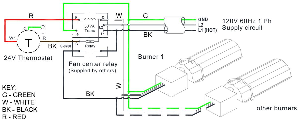
**⚠ If any of the original wire as supplied with the appliance must be replaced, it must be replaced with wiring material having a temperature rating of at least 220°**
