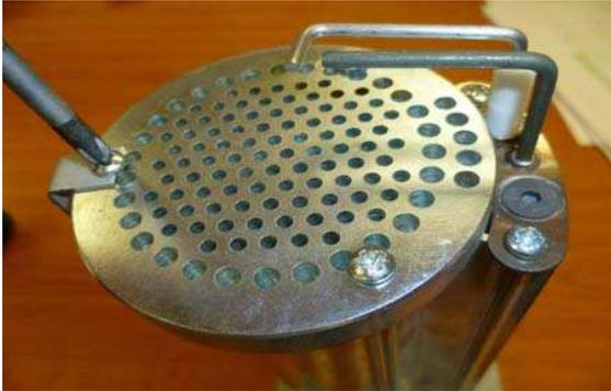
**Step 2:** The pepper pot burner head can be replaced ensuring the 5 holes on the outer ring are aligned alongside the probes.
