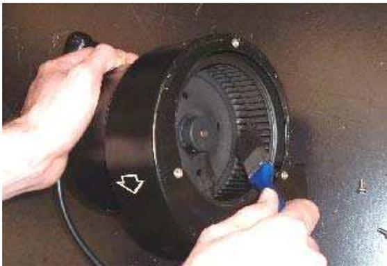
**Step 6:** Remove any dust from fan scroll and from around the motor.
