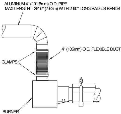
**Figure 6.d Wall Terminal Intake Kit.**
