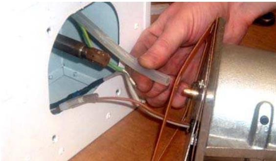
**Step 6:** Detach the two screws holding the front of the gas valve.
