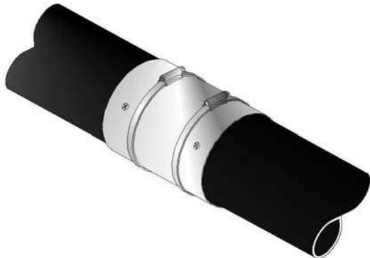
Slide the coupler over the tube ensuring that the tube stop has butted up to the tube ends. Using a 5/16" drive or flat blade screwdriver, tighten the bolts.
