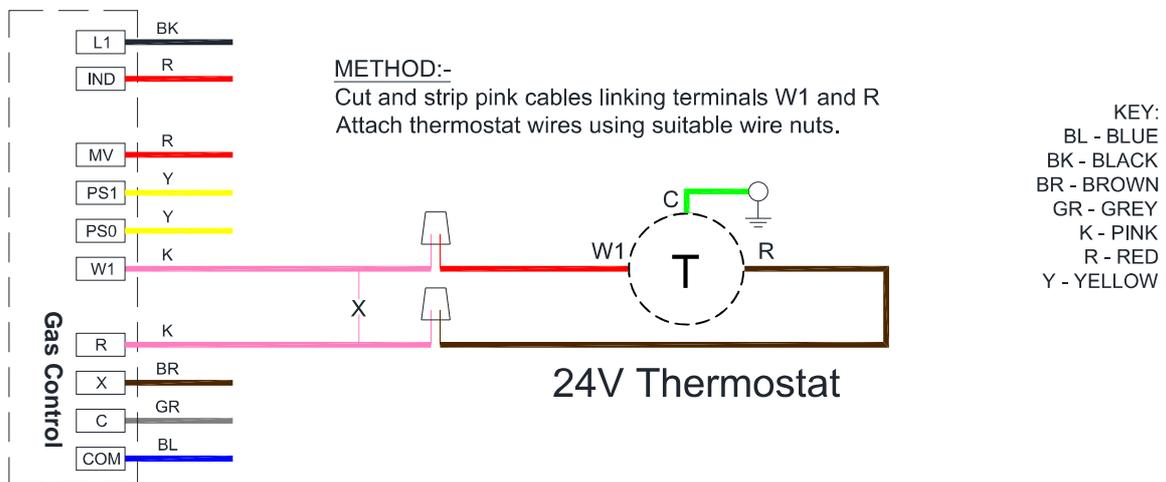
**Figure 5e. Multiple Heater Installations 24V Control**
