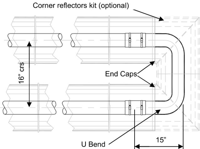
**!** Bends must be fitted at a distance of at least 50% of the total heat exchanger e.g. for a 60ft long heater, the closest to the burner a bend can be is 30ft.
