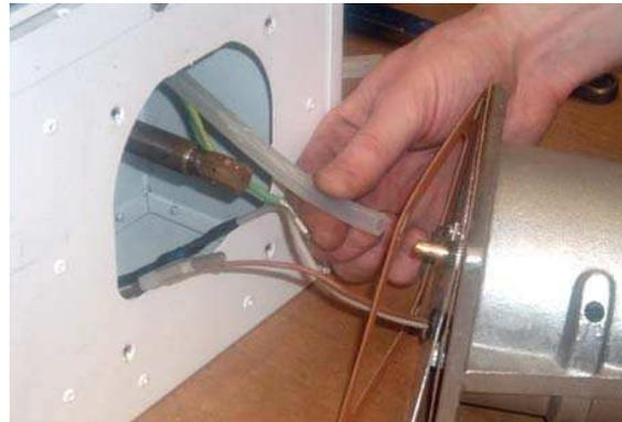
**Step 2:** The gas injector can be inspected and replaced if contaminated or blocked.
