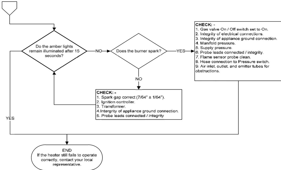
To aid the troubleshooting process, the UT controller has a LED flash code diagnostic sequence:
