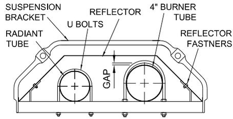
FIRST POINT SUSPENSION BRACKET TYPE A
