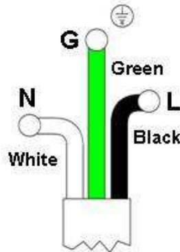
**Figure 5.a Typical U-Tube Range Wiring Connections**
