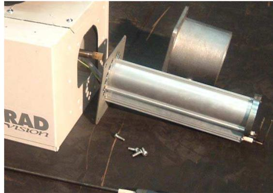
**Step 1.b:** The burner head assembly can be disconnected by separating the connectors of the ignition lead assembly and removing the pressure switch silicon tube.
