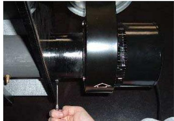
**Step 3:** The combustion fan can now be detached.
