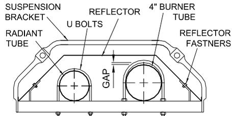
FIRST POINT SUSPENSION BRACKET TYPE A
