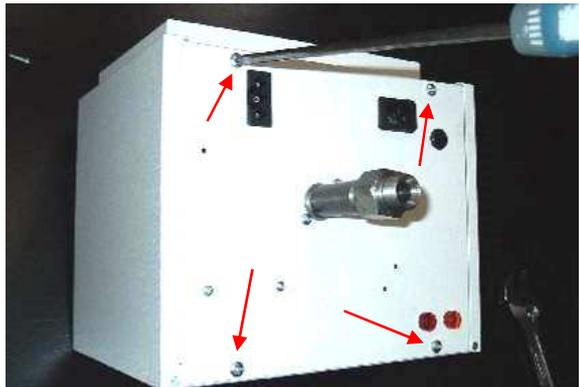
**Step 8:** Remove the rear plate complete with gas fitting .
