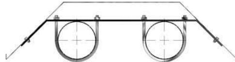
Slip the brackets onto the tubes in correct order and fix at correct points as shown on the relevant assembly drawing. Ensure fixings are tight to brackets
