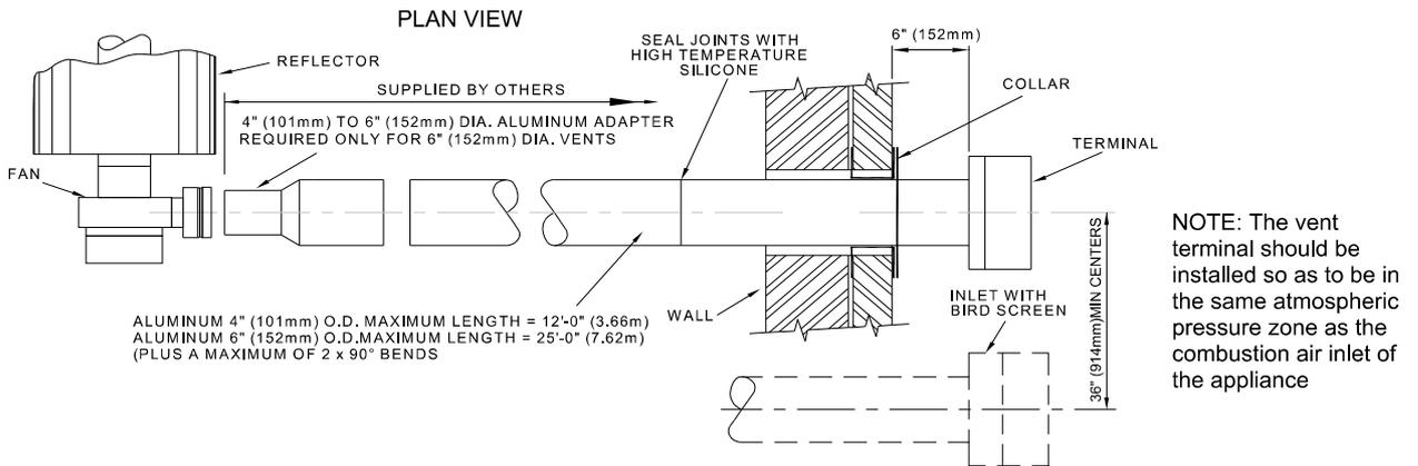
**Figure 6.c Fresh Air Ducted Intake.**
