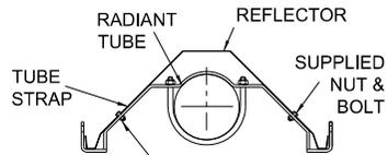
2 x SCREWS TIGHTEN TO FIX REFLECTOR
