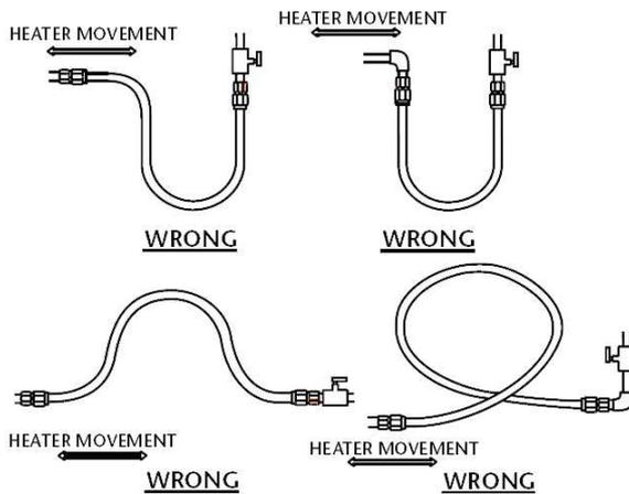
**WARNING: FIRE OR EXPLOSION HAZARD** - Expansion of the radiant pipe occurs with each firing cycle causing the burner to move with respect to the gas line. This can result in a gas leak producing an unsafe condition. It is therefore essential to provide some flexibility in the final gas line connection by use of an approved armoured flexible connector or stainless steel expansion loop as shown in the drawings.
