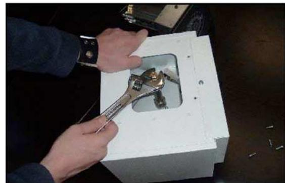
**Step 3:** Reconnect ignition leads and silicon tube to test nipple. Refit gasket and support casting.
