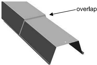
Slide the next reflector backwards through the brackets and **overlap** the existing reflector until the locating slots line up with the type 'F' reflector support bracket.
